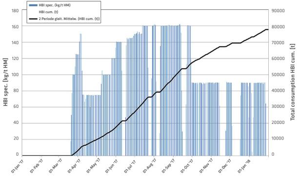
FIGURE 4. HBI quantity used in BF operation
