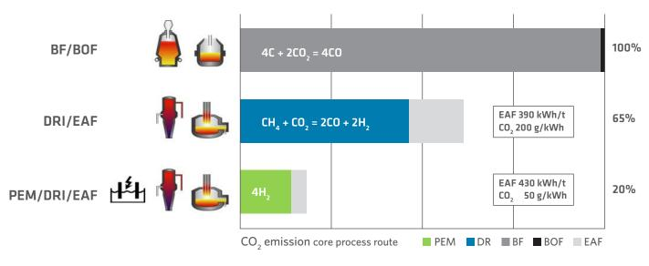
**FIGURE 2.** CO<sub>2</sub> emissions of steel production routes
