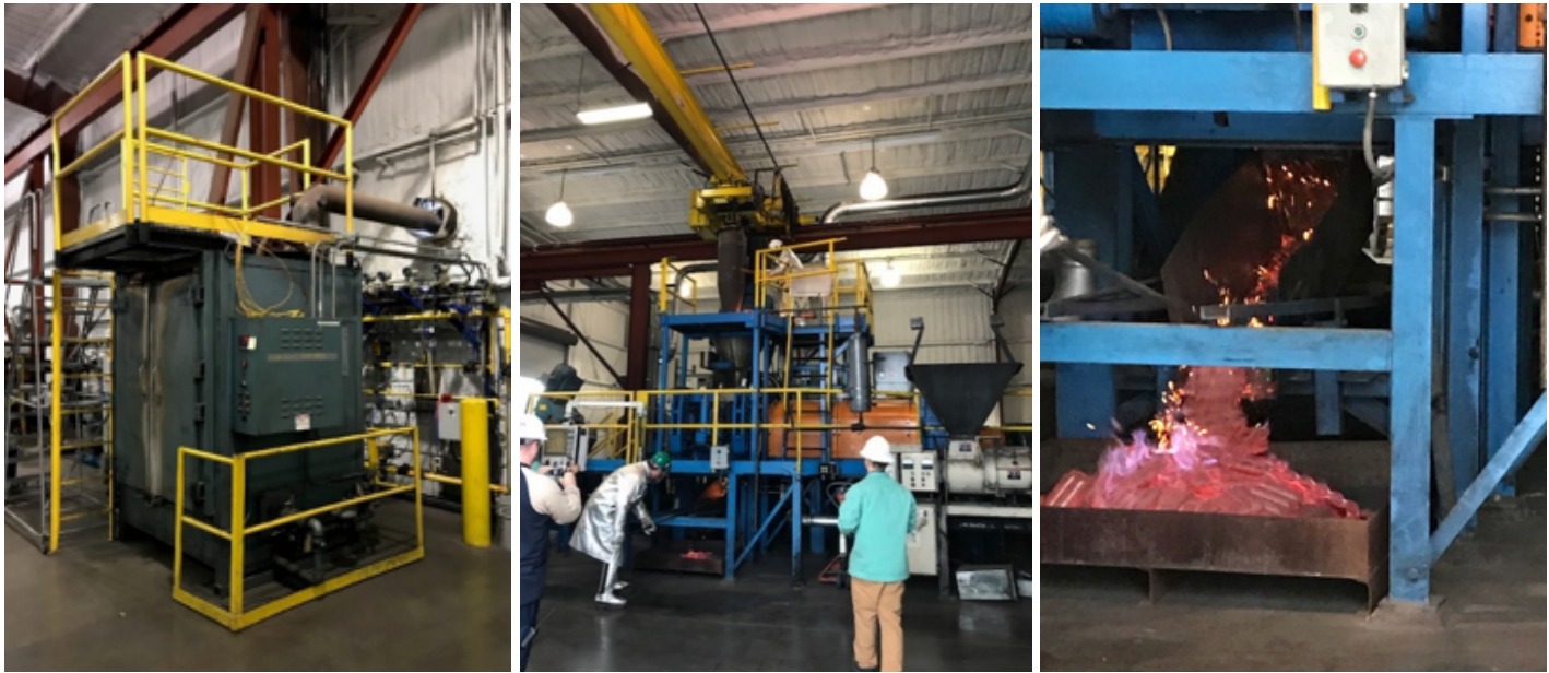
FIGURE 7. Large reduction furnace and HBI coming off the Köppern press
