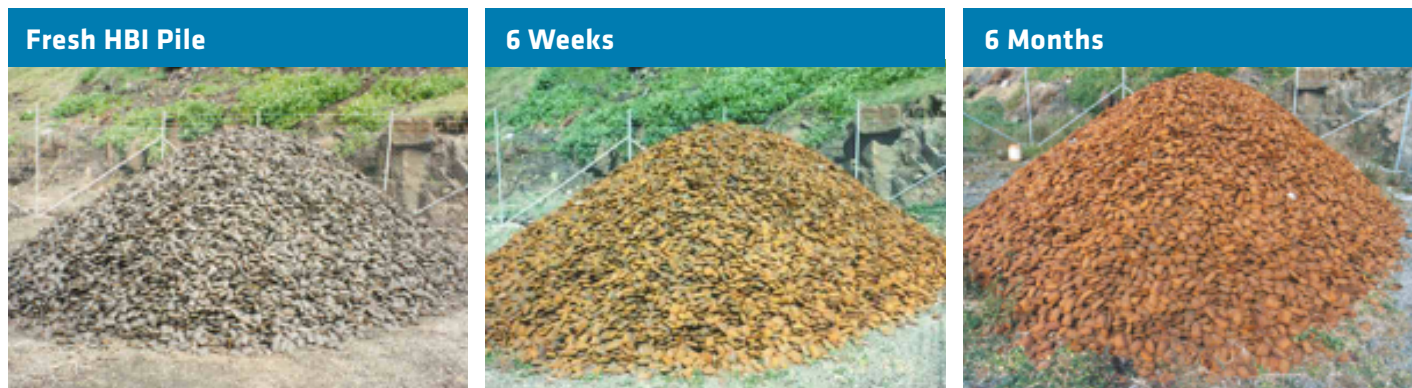
FIGURE 5 HBI corrosion test pile (courtesy of BHP Billiton)
