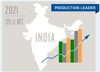
ndia continued its streak as the number one DRI producer worldwide, producing a record 39.11 Mt of DRI - 30.11 Mt in rotary kilns and 9.00 Mt by gas-based processes - a 18.6 % increase overall, one of the highest growth rates in the history of the Indian DRI industry. According to the Sponge Iron Manufacturers Association (SIMA) of India, rotary kilns saw a 18.8% increase from 2020, after a 27.9% increase from 2018 to 2019, following a 35% increase from 2017. Production
