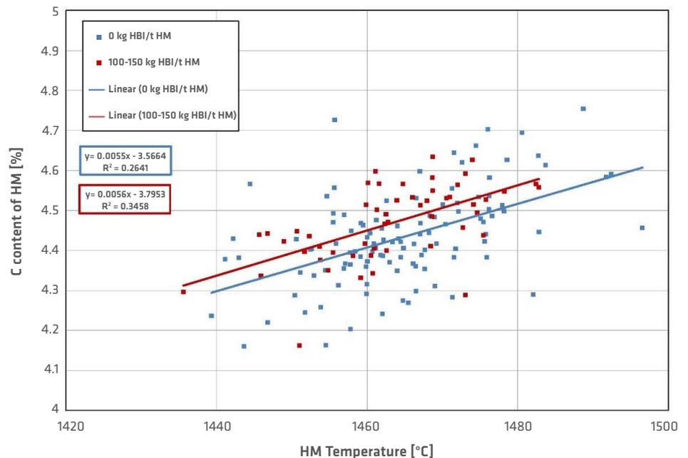
FIGURE 9. Carbon content in hot metal
