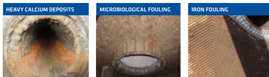
FIGURE 2. Typical problems found in DRI plant water system
