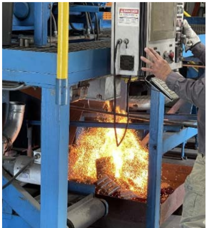
FIGURE 2. Commercial-scale HB machine and the discharged HBI at Midrex R&D Center
