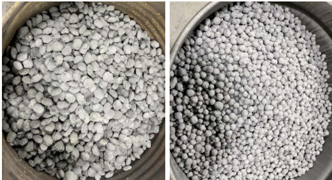
FIGURE 1. Composite DRI samples for CBQ-DRI (left) and pellet-DRI (right)
