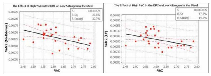
FIGURE 1 Effect of High %C on the Nitrogen content at meltdown and at the Ladle Furnace.
