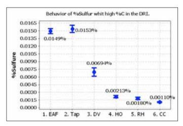
FIGURE 5 Sulfur content in each process stage for steelmaking.
