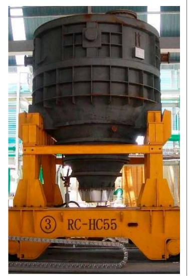
FIGURE 2 Hot Transport Vessel at LION
