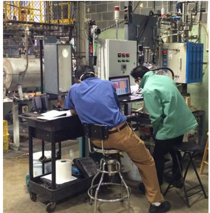
FIGURE 2. Test stand at Midrex R&D Center used to verify the ACT ™ concept and to perform experiments that provided the data needed to develop the commercial design.
