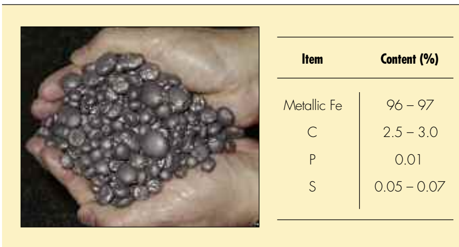
Figure 9 - Photo and chemical analysis of iron nuggets
