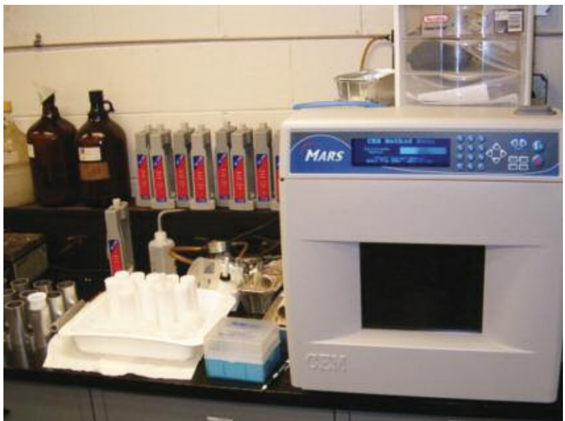
Figure 5 - Microwave Digestion for the ICP
