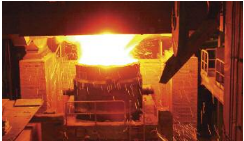
Figure 4 - Qatar Steel: Molten Steel Tapping at EAF2R
