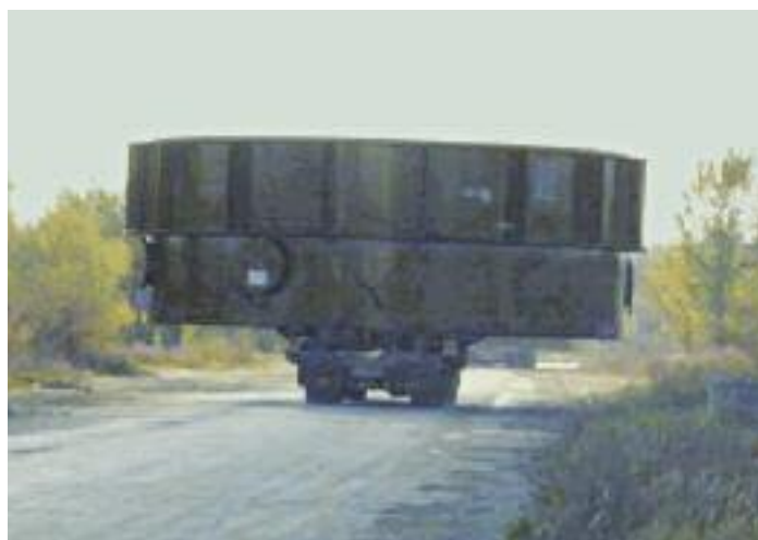
Figure 3 - Shaft Furnace Casing Being Delivered
